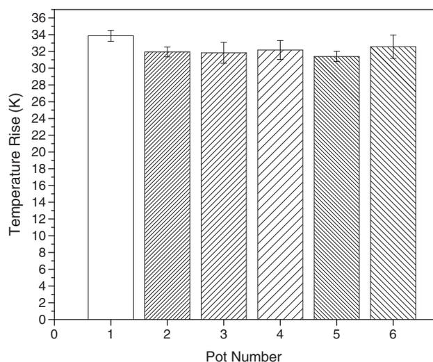
**Fig. 9.** Effect of pot geometry and material on heat transfer to a cooking pot. Uncertainty bars represent one standard deviation.
