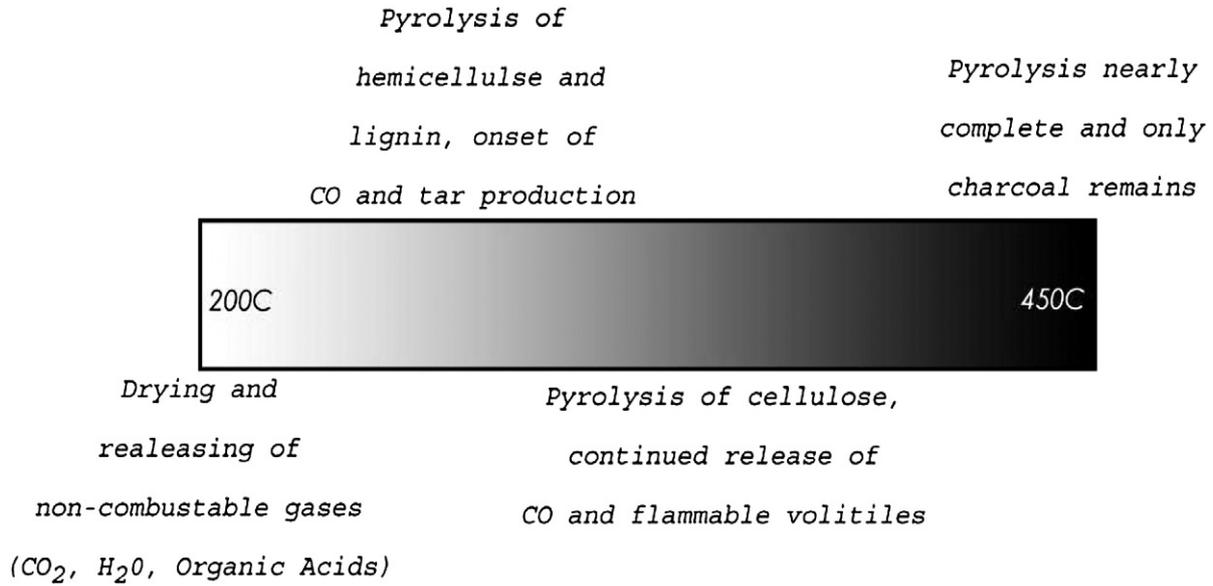
Fig. 1. Stages of wood combustion and associated chemical compounds with respect to increasing temperature.
