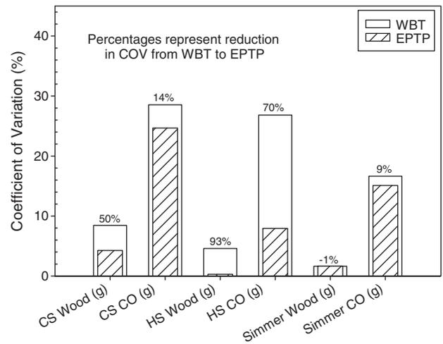
Fig. 11. Coefficients of variation following the WBT and EPTP Methods.
