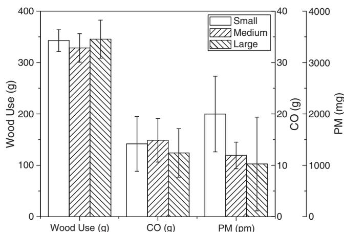
Fig. 4. Effect of fuel size on wood use, carbon monoxide, and particulate matter. Uncertainty bars represent one standard deviation.
