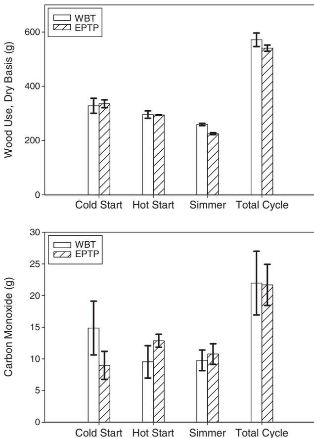
Fig. 10. Stove performance following the WBT and EPTP Tests. Uncertainty bars represent one standard deviation.
