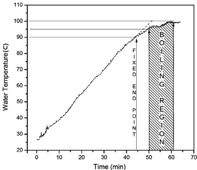
Fig. 2. Ambiguity of boiling point due to slight variations in vaporization temperature.
