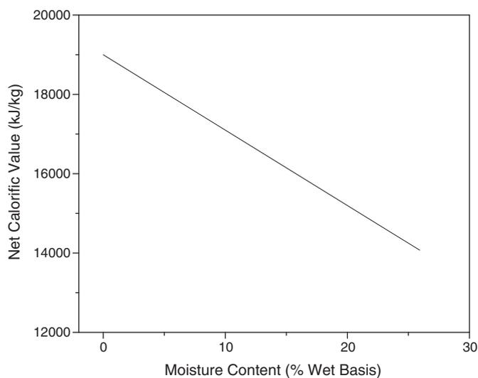
Fig. 5. Effect of moisture content on net wood calorific value (Van Loo and Koppejan, 2008).
