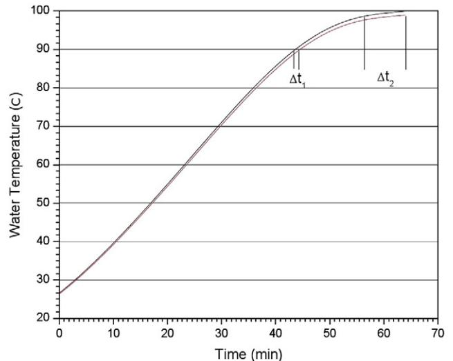
Fig. 3. Uncertainty in test duration due to slight variations in water boiling point.
