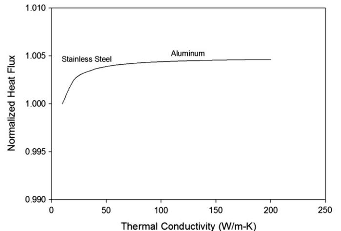
Fig. 8. Influence of pot conductivity on heat flux into water.
