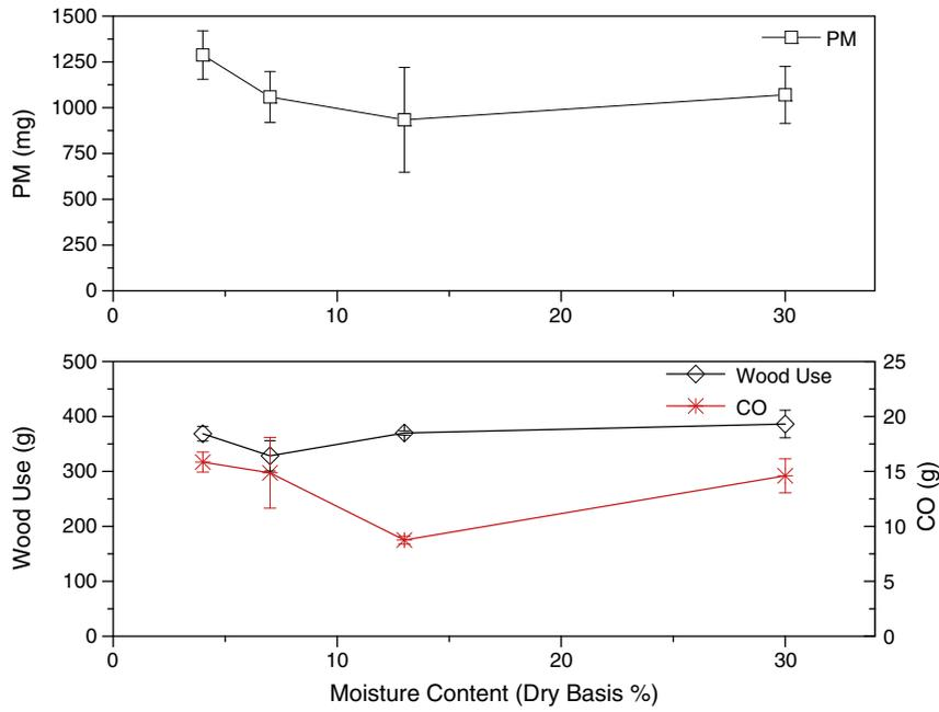
Fig. 6. Effect of changing moisture content on stove performance. Uncertainty bars represent one standard deviation.
